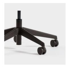
The five-star base used on Max contains a steel ring to help support the height adjustment spindle. Traditionally this was moulded into the plastic base, but was difficult to extract at the end of life, making recycling much more challenging. The Max five star base still contains the steel ring, but we have re-designed the base so that the steel ring can be easily removed, allowing the plastic base and the steel ring to be easily separated and then recycled at the end of life.
